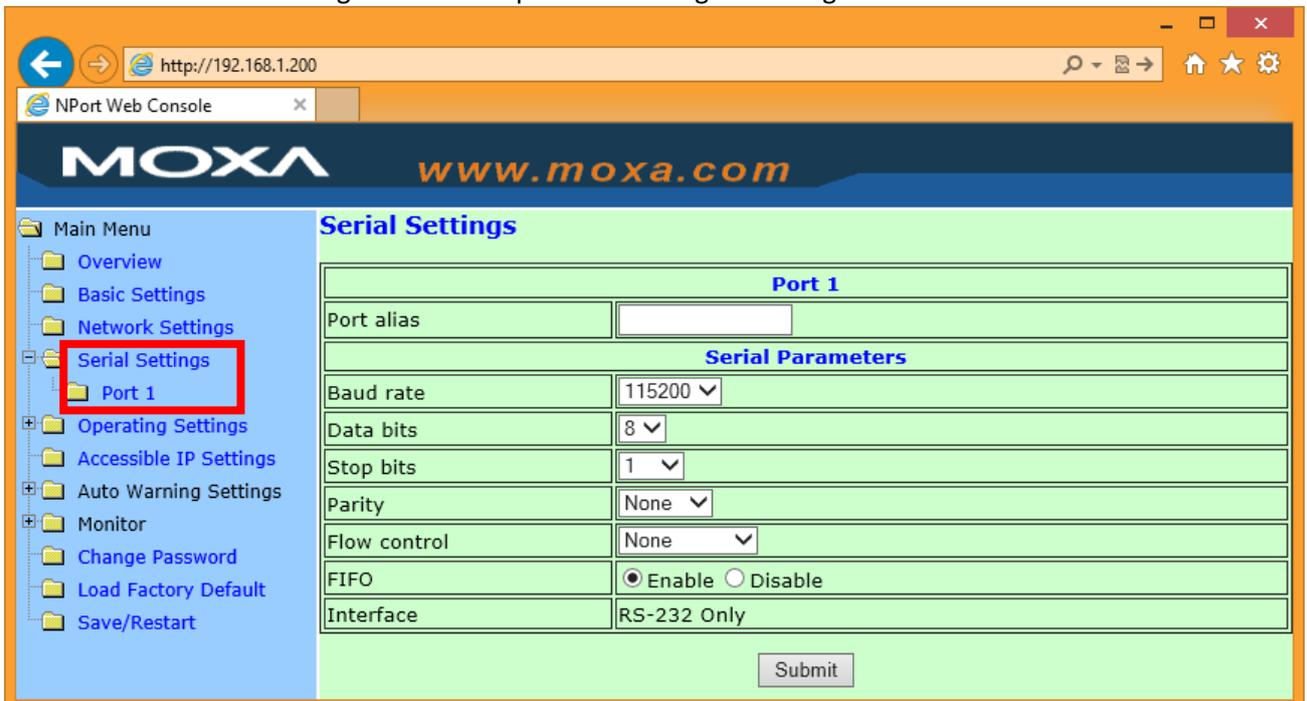
The screenshot shows the MOXA NPort Web Console interface. The left sidebar contains a 'Main Menu' with 'Serial Settings' and its sub-item 'Port 1' highlighted with a red box. The main content area is titled 'Serial Settings' and shows configuration for 'Port 1'.
